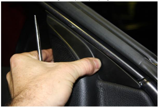
Remove door trim with firm pulling action starting at the bottom using the lower pocket as leverage
