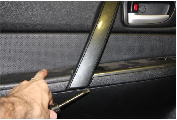
Remove light cover with firm pulling action and undo one screw inside
