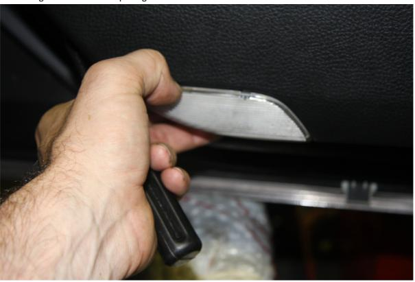
Remove inner handle screw cover by prying with flat head screwdriver and undo one screw
