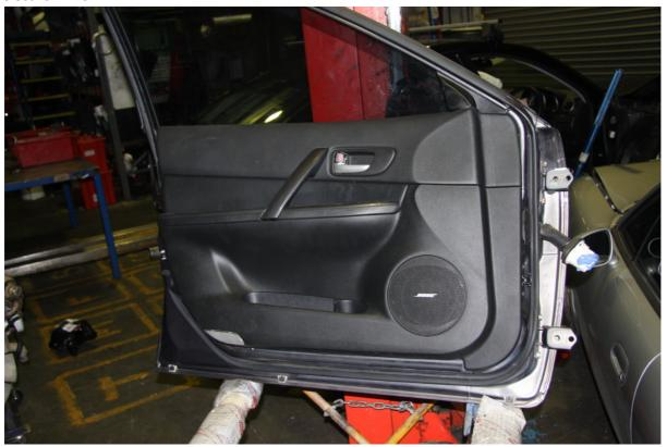
Remove trim piece in grab handle by levering with screwdriver then remove two screws
